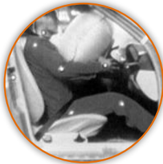
Stages of the driver airbag performance during an accident
